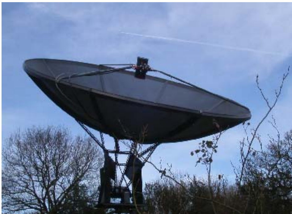
Figure 2 - 3m' Dish with 1420MHz Cylindrical Waveguide Feed
